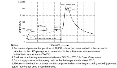
6 No more than one wave soldering pass.
