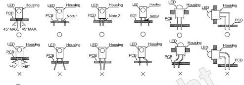
" ( ) " Correct mounting method " imes " Incorrect mounting method
