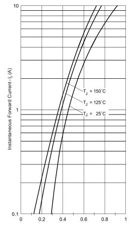
Forward Voltage Drop -  $V_{_{FM}}(V)$  Fig. 1 - Maximum Forward Voltage Drop Characteristics
