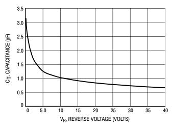
Figure 3. Typical Capacitance
