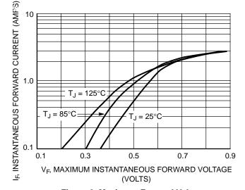
Figure 2. Maximum Forward Voltage
