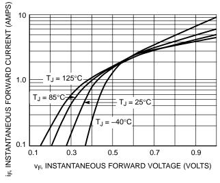
Figure 1. Typical Forward Voltage
