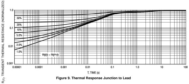
Figure 9. Thermal Response Junction to Lead
