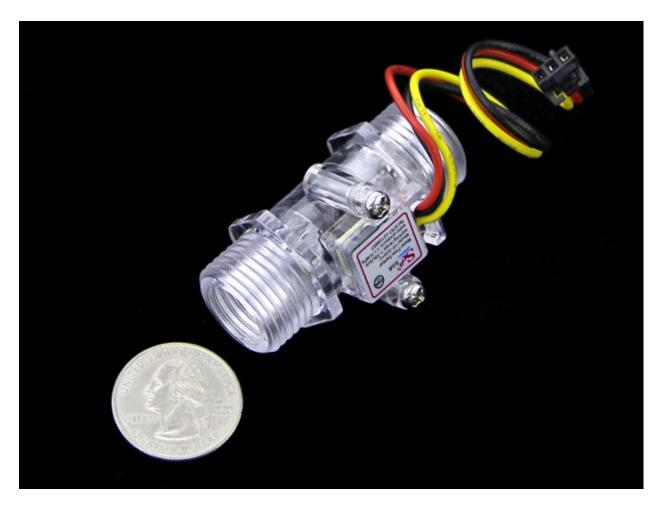
Water flow sensor consists of a plastic valve body, a water rotor, and a hall-effect sensor. When water flows through the rotor, rotor rolls. Its speed changes with different rate of flow. The hall-effect sensor outputs the corresponding pulse signal. This one is suitable to detect flow in water dispenser or coffee machine.
